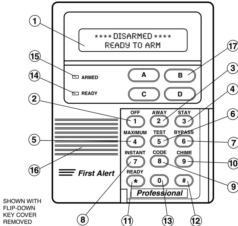
**IMPORTANT!:** When using the keypad to enter codes and commands, sequential key depressions must be made within 3 seconds of one another. If 3 seconds elapses without a key depression, the entry is aborted and must be repeated from its beginning.
