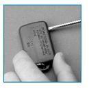
2. Place the case, buttons down, on work surface. Remove case back by inserting the blade of a small flat head screwdriver into the seam around the case and prying the case open. Leave the circuit board assembly in the case front, buttons down.
